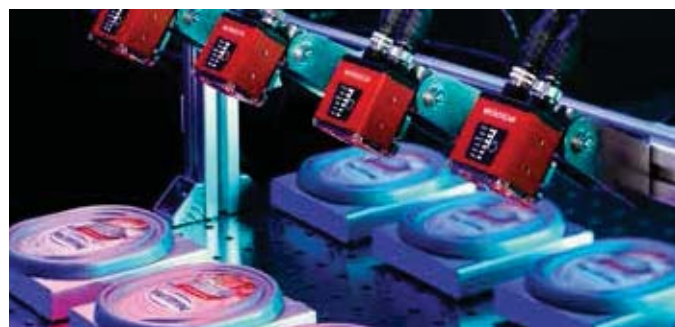
Omron's MicroHAWK series of industrial barcode readers enhance traceability and flexible manufacturing with best-in-class liquid lens autofocus technology, including new long range functionality, and high-performance X-Mode decoding algorithms.
